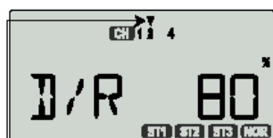
Upper arrow indicates upper D/R switch setting
